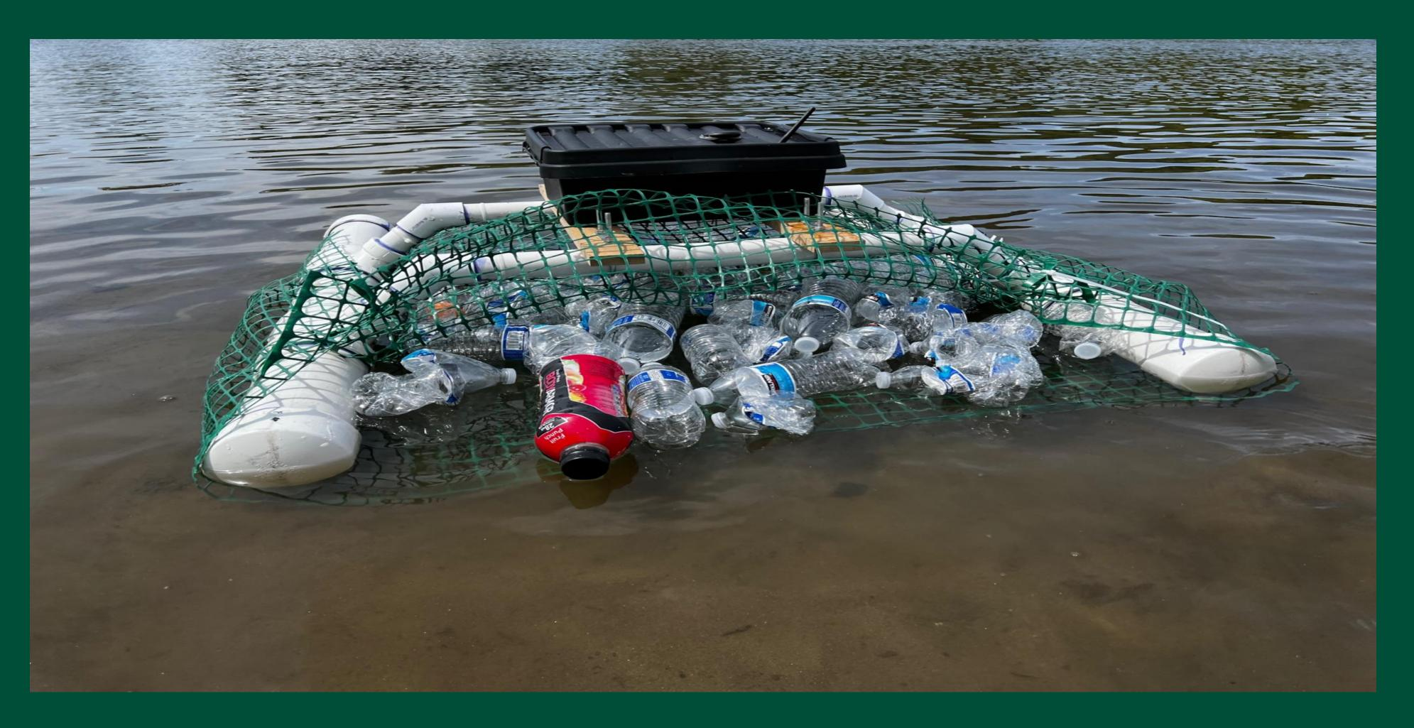
Figure 1: Image of Plastic Collecting Rover
